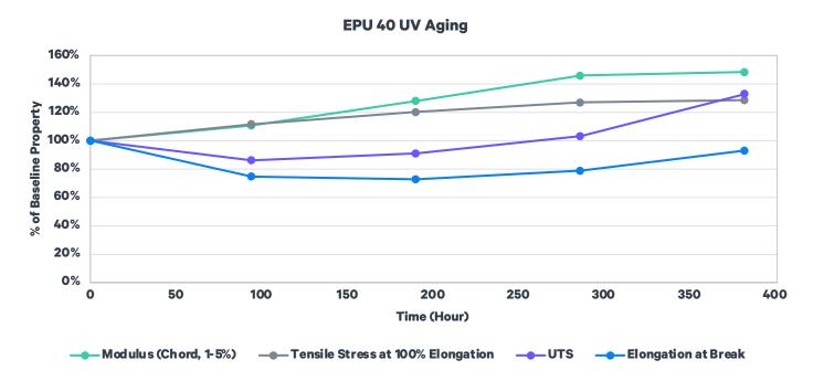
ASTM D4459: Q-Sun XE-1, 0.8 W/m²/nm at 420 nm, 55  $^{\circ}$ C ASTM D412: Die C, 500 mm/min, average values represented
