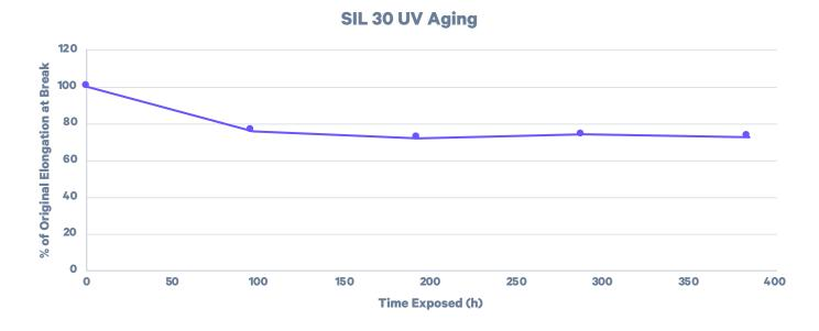
ASTM D4459: Q-Sun XE-1, 0.8 W/m² at 420 nm, 55  $^\circ \rm C$  ASTM D412: Die C, 500 mm/min, average values represented
